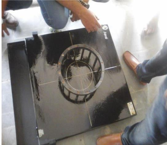
**Fig: 4.2 J - ring test Apparatus**
