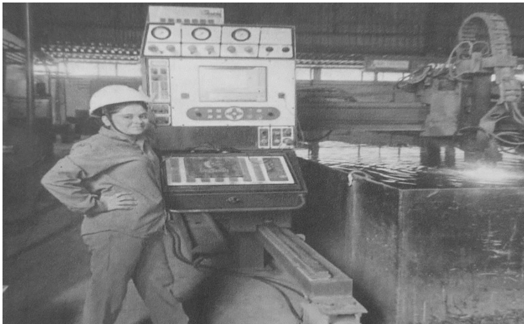
Fig 5.1 Woman operating CNC plasma cutting machine
