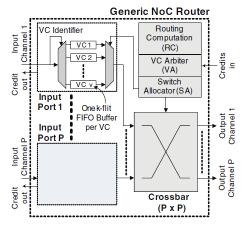
Figure 2. Generic NoC router architecture.
