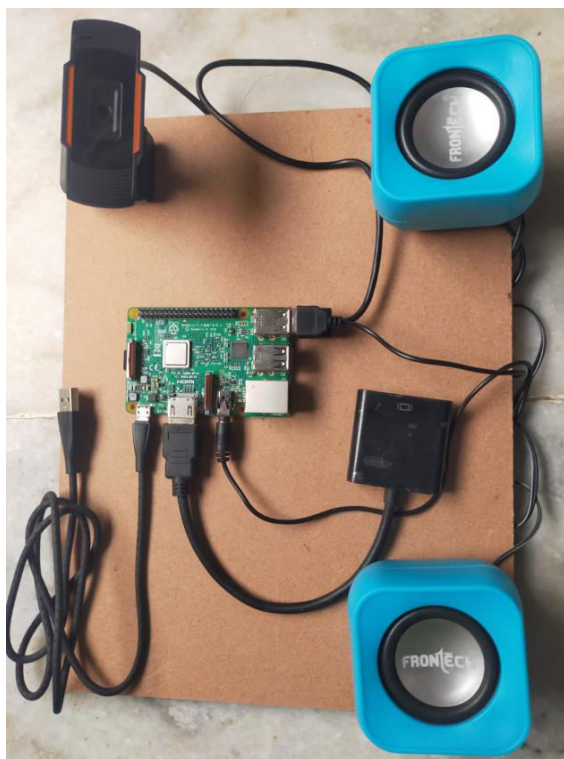
Fig.4. Hardware setup of smart electronic vehicle surveillance system
