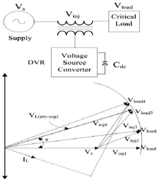
Fig. 1. (a) Basic circuit of DVR, (b) Phasor diagram of the DVR voltage injection schemes.
