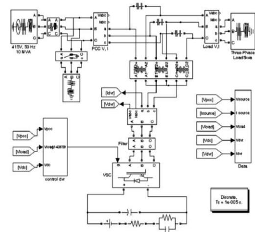
Fig. 5 MATLAB based model of the BESS supported DVR connected system.
