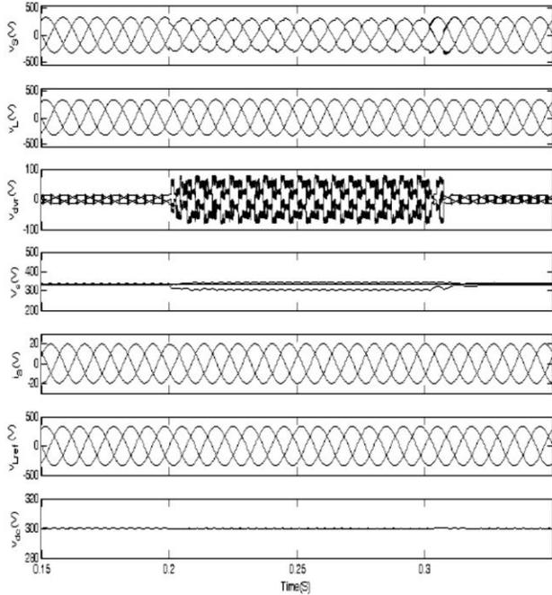
Fig. 8. Dynamic performance of DVR during harmonics in supply voltage applied to critical load.
