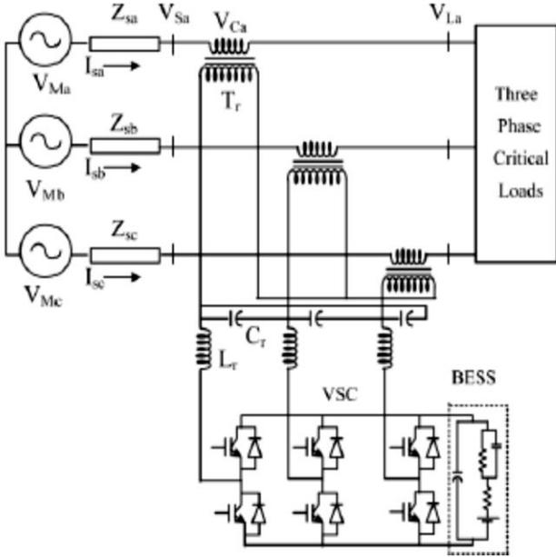
Fig. 2. Schematic diagram of the DVR connected system.
