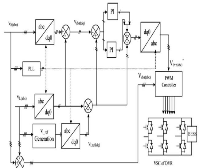
Fig. 3. Control block of the DVR which use the SRF method of control.
