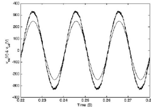
**Fig. 7. Voltages at PCC and Load terminals.**
