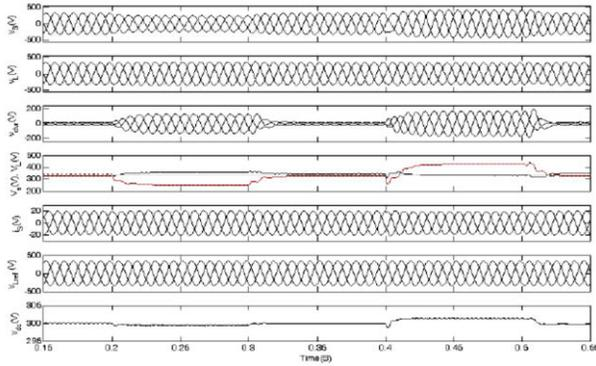
**Fig. 6 Dynamic performance of DVR with inphase injection during voltage sag and swell applied to critical load.**
