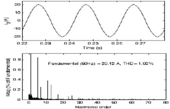
Fig.10. Supply current and harmonic spectrum
