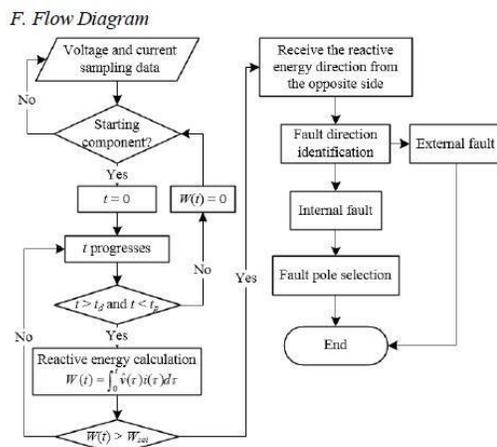
Fig.5 Flowchart of protection scheme
