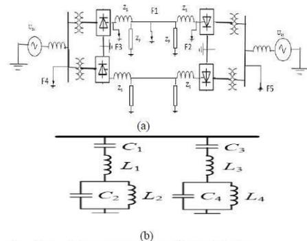
Fig.1 (a) Equivalent HVDC system (b) DC side filter
