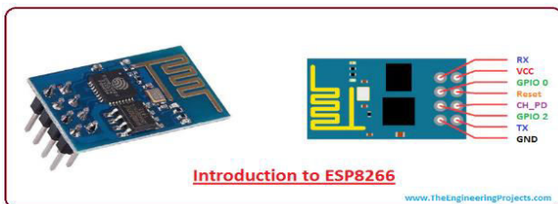
Fig 8 representation of the parts of ESP8266
