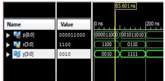
Fig.9 Simulation of Systolic multiplier in radix-binary
