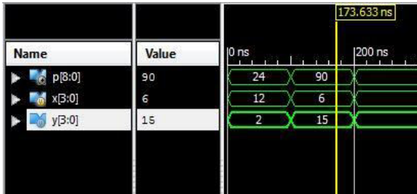
Fig.10 Simulation of Systolic multiplier in radix-decimal
