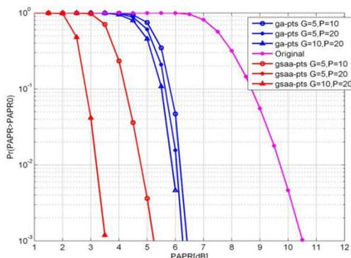
Fig 3 : Comparison of PAPR CCDF of GA-PTS and GSAA-PTS with 128 subcarriers
