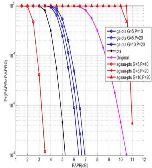
Fig 4: Comparison of PAPR CCDF of GA-PTS and AGSAA-PTS with original PTS having 128 subcarriers
