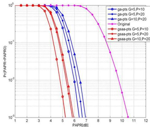
Fig 2 : Comparison of PAPR CCDF of GA-PTS and GSAA-PTS with 64 subcarriers
