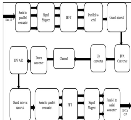
Fig. 1: Block diagram of OFDM signal
