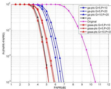
Fig 4: Comparison of PAPR CCDF of GA-PTS and GSAA-PTS with original PTS having 64 subcarriers
