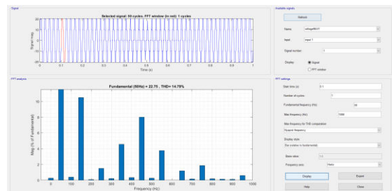
Fig.22 THD% of voltage
