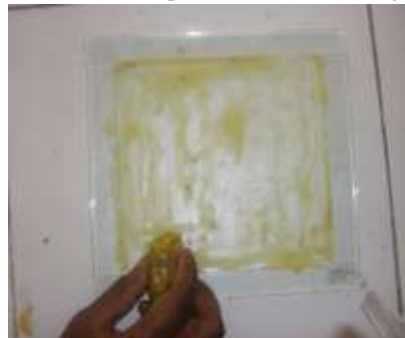
Fig: 2.3 applying Wax to the mould
