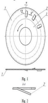
The device works as follows. When the saw cylinder rotates, its surface creates an air flow that rotates with the saw cylinder. This air flow, when it meets the air flow that goes along the technological chain of cotton processing from the gin branch pipe, are connected (the previous
