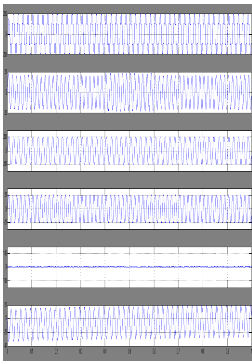
Fig.9. Simulation waveforms for voltage swell. (a). Source Voltage V_s , (b). Source current i_s , (c). load voltage V_L , (d) load current i_L , (e) Active-filter voltage V_{comp} , and (f) Harmonic current of the passive filter i_{PF} .
