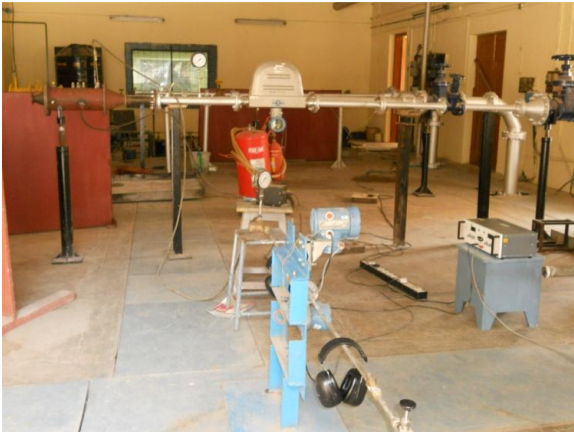
Figure.5 Experimental setup of can-combustor testing
