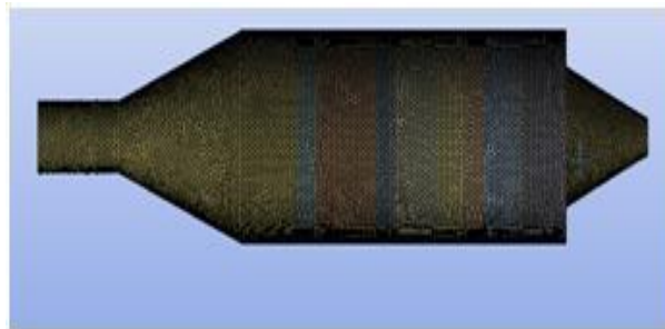
Figure.3 CFD meshing domain designed for can-combustor
