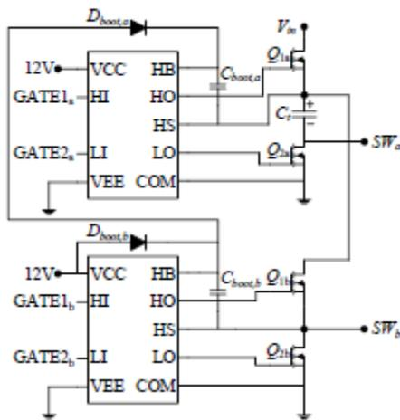
Fig. 11. Gates drivers' realization in the TIFLLC converter.
