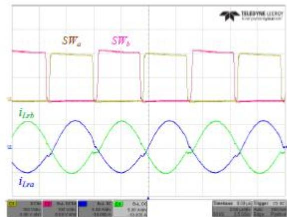
Fig. 14. Experimental waveforms of the TIFLLC converter. C1 – switching node voltage of phase *a*  $SWa(100V/div)$ , C2 – switching node voltage of phase *b*  $SWb(100V/div)$ , C3 – phase *a* primary-side resonant tank current  $iLra(5A/div)$ , C4 –
