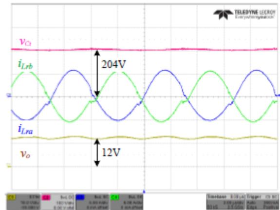
Fig. 12. Experimental waveforms of the TIFLLC converter. C1 – output voltage  $v_o$ (5V/div), C2 – flying-capacitor voltage  $v_{Ct}$ (100V/div), C3 – phase  $a$  primary-side resonant tank current  $i_{Lra}$ (5A/div), C4 –
