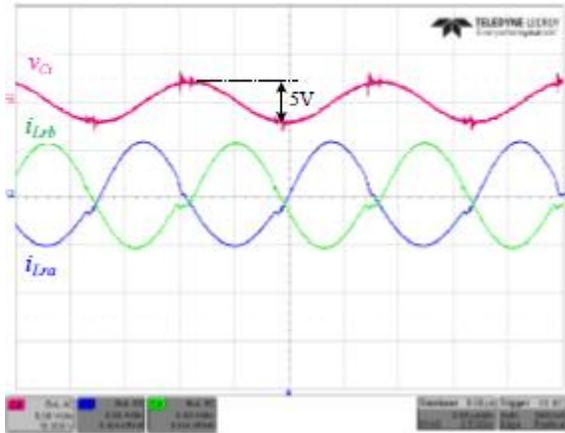
Fig. 13. Experimental waveforms of the TIFLLC converter. C2 – flying-capacitor voltage  $vCt(5V/div, ac\ coupled)$ , C3 – phase *a* primary-side resonant tank current  $iLra(5A/div)$ , C4 – phase *b* primary-side resonant tank current  $iLrb(5A/div)$ . Time scale is  $2\mu s/div$ .
