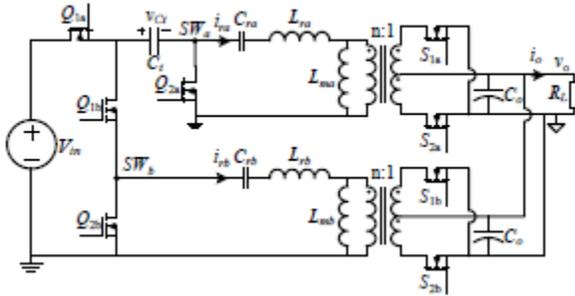
Fig. 1. Two-phase interleaved flying-capacitor LLC (TIFLLC) converter topology.
