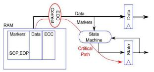
Fig. 1. Typical packet data storage in a networking application.
