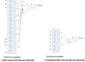
Fig. 2 Decoding of a control bit for single and independent SEC codes for data and control. (a) SEC code for both data and control bits. (b) Independent SEC codes for data and control bits.
