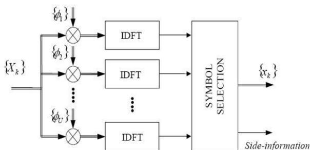
**Fig 1 : Scheme of a Modulator with Selective Mapping**
