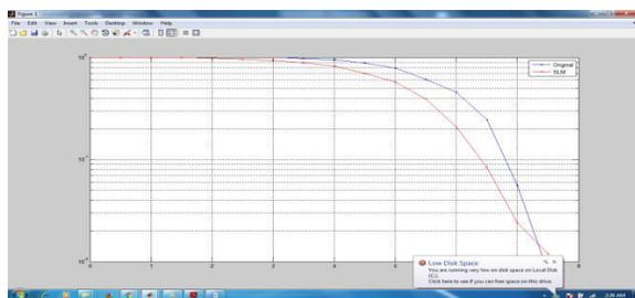
Fig 5.CCDFs of SLM for OFDM PAPR reduction
