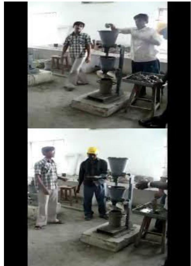
Compaction factor measures the workability in an indirect manner by determining the degree of compaction achieved by a standard amount of work done by allowing the concrete to fall through a standard height.
