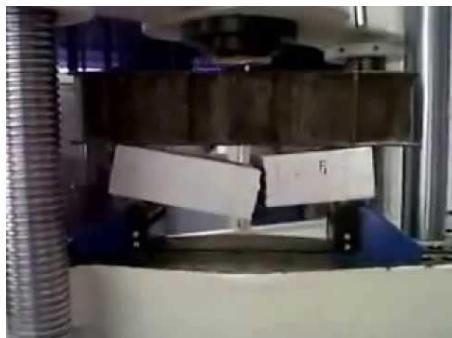
In the flexural strength test theoretical maximum tensile stress reached at the bottom fibres of the test beam is known as the modulus of rupture. When concrete is subjected to bending stress, compressive as well as tensile stresses are developed at top and bottom fibres respectively. The strength shown by the concrete against bending is known as flexural strength. The standard size of specimen is 100mm×100mm×500m with a span of 600mm.
