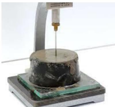
Lower the needle gently and bring it in contact with the surface of the test block and quickly release. Allow it to penetrate into the test block.
