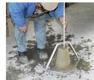
Slump test is the most commonly used method of measuring consistency of concrete which can be employed either in laboratory or at site of work.
