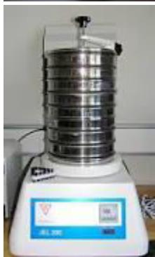
The process of dividing a sample of aggregates into fractions of same particle size is known as a sieve analysis and its purpose is to find fineness. The sieve analysis was carried out using locally available river sand and tabulated in table 3.5.
