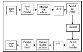
Fig 1: Block Diagram of FFT Based OFDM System
