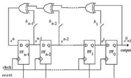
Fig.5: Simplified circuit of a generic LFSR circuit
