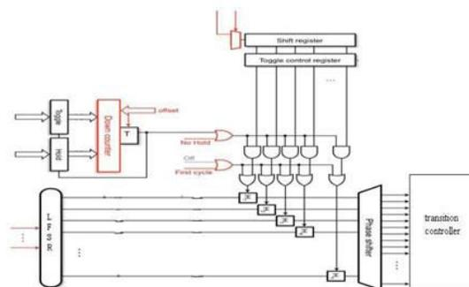
Fig 4: LP decompressor with LFSR and transition controller
