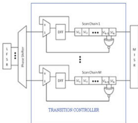
Fig 6: Low power PRPG with transition controller
