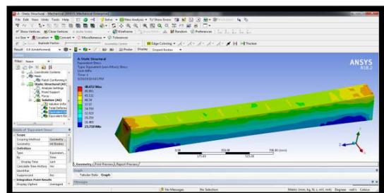
Fig 4.17 Stress of light weight concrete
