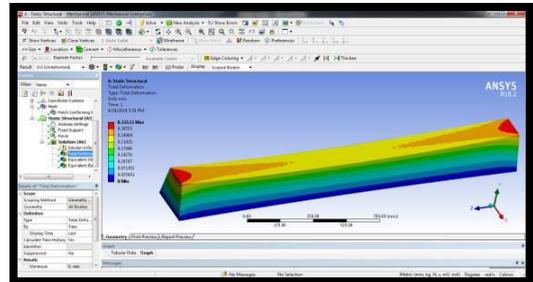
Fig 4.14 Deformation of concrete
