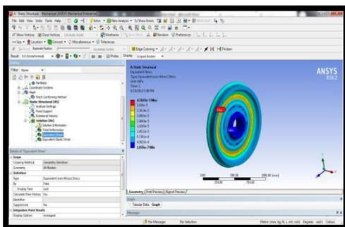
Fig 4.13 stress of nickel chromium molybdenum alloy steel
