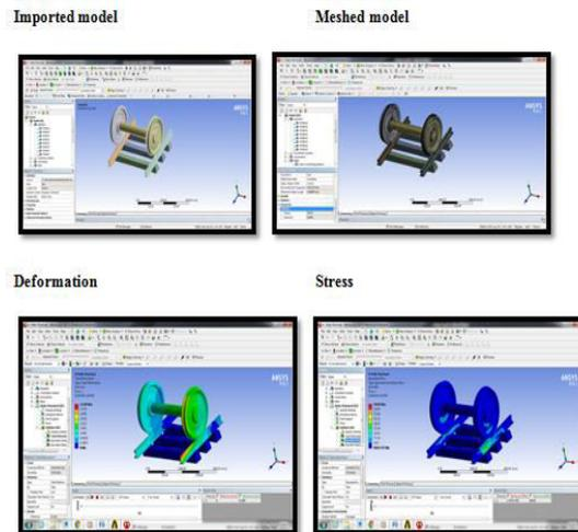
**Fig 4.18 STATIC ANALYSIS OF ASSEMBLY OF RAIL WHEEL**
