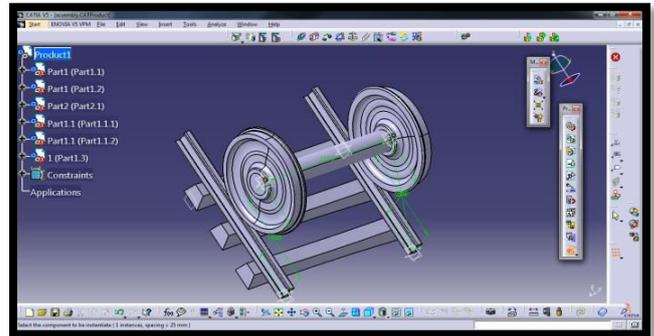
Fig 4.7 assembly of rail wheel
