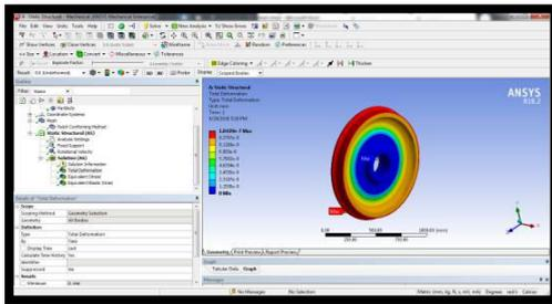
Fig 4.10 Deformation of high carbon steel
