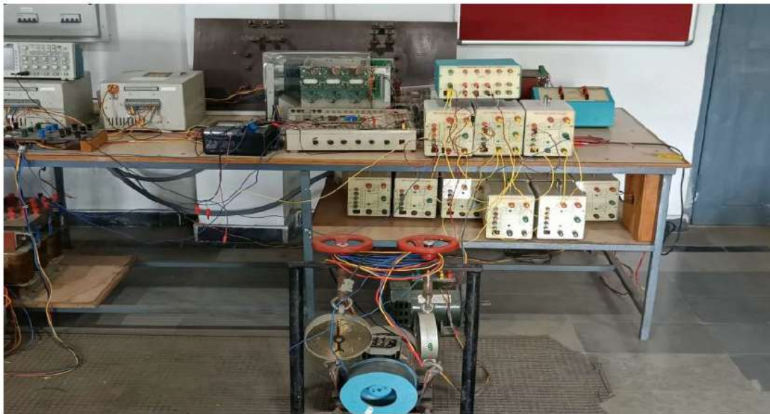
Fig. 11. Experimental setup of the FPGA-controlled induction motor drive.
