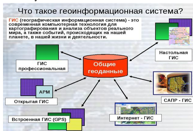
Fig.1. General geodata of GIS technologies.
