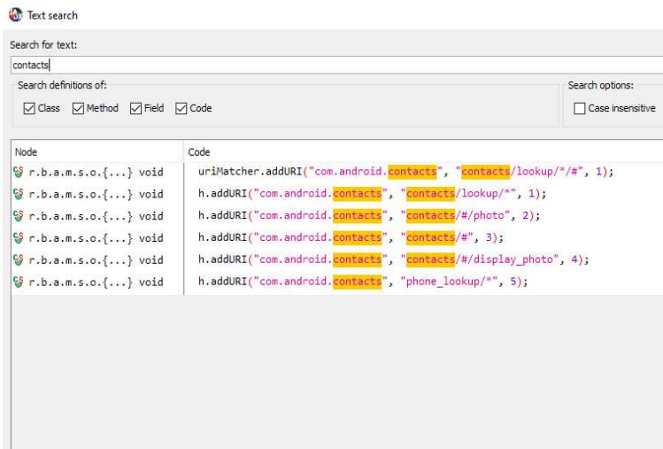
Figure 2.8: penetration test result showing app accessing the contact list from the device
